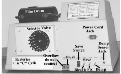
5. OVERFLOW - DO NOT CONNECT. If solution comes out of this outlet, check your FLUSH tubing for proper installation.
