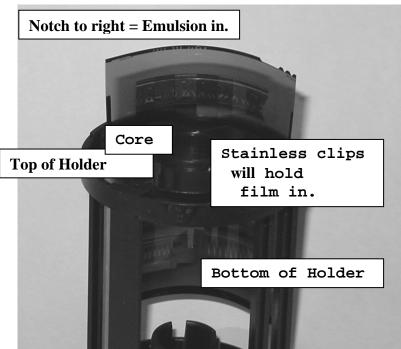
Select DRUM SIZE = 4 for 1 HOLDER in the 4-roll DRUM and DRUM SIZE = 6 for 2 HOLDERS in the 8-roll DRUM.
