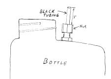
both ends of the tubing with the chemical name. Slip one end over the proper tube and the other end over the exposed black tubing of the solution bottle. Use the 7 liter Bottle Template to make volume marks on the bottle. The 5 gal. Water bottle connects to the WATER (#5) tube.
