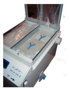
STOP ends the thawing and drains the bladders.
