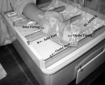
Mount the BLADDER by pushing the INLET and OUTLET FITTINGS down and twisting back and forth on the INLET and OUTLET PORTS. Slip on the GROMMETS over the studs in the LID. If you are not using all 3 BLADDERS you must cover any open INLET (larger) ports with a plug.
