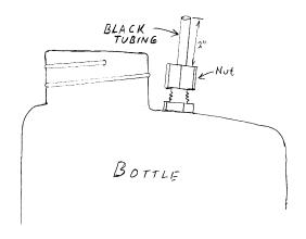
DOWN from the back of the machine. After about a foot, the tubing can run in any direction Allow about 2 feet (60 cm.) extra for slack. Label both ends of the tubing with the chemical name. Slip one end over the proper tube and the other end over the exposed black tubing of the solution bottle. The 5 gal. water bottle connects to the WATER (#5) tube.
